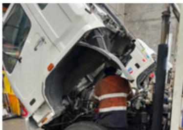
We removed engine components on this Mitsubishi Fuso Fighter to repair oil leaks and restore efficiency.
